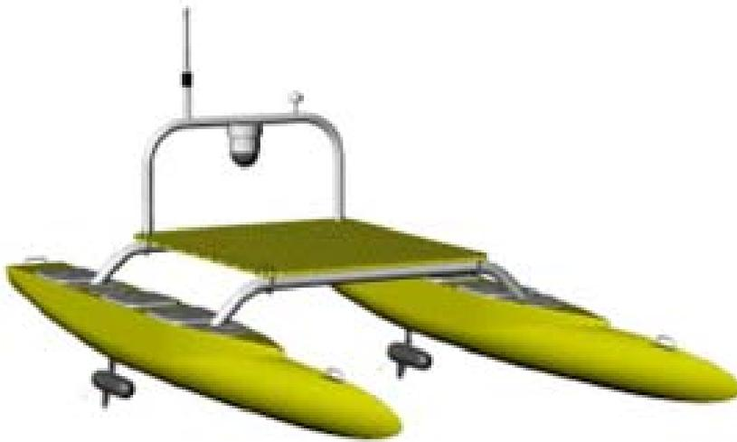
Figure 2: NURC's Autonomous Surface Vehicle (ASV)
