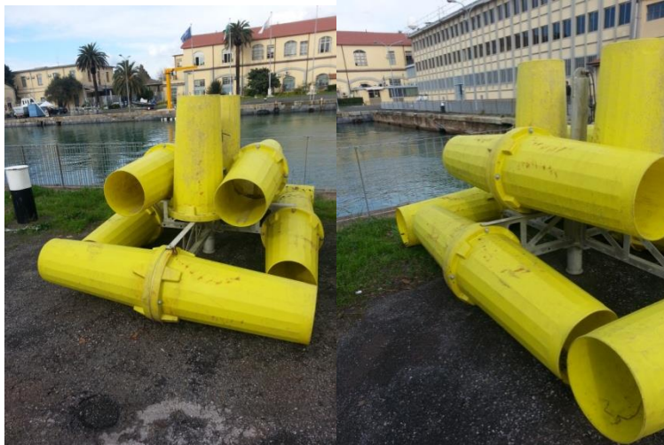
Fig. 5. Piping assembly structure used in SAUC-E 2016. (Left) Frontal view. (Right) Lateral view. The structure, composed of yellow pipes, has the following dimensions: 2 m (front area) x 3 m x 1.8 m (height).
