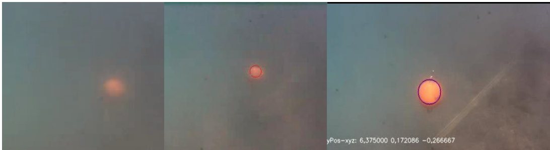
Figure 4b: SAUC-E 2011 Bremen's buoy servoing: detection, initial lock on it, final tracking and circling around it. This will be an anomaly for Task 3 in SAUC-E'16.
